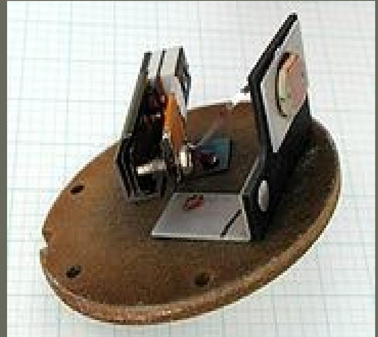
**The internal components of a photoelectric control for a typical American streetlight.**
