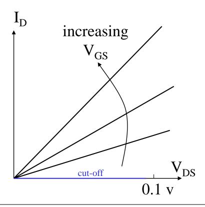
Increasing V<sub>GS</sub> puts more charge in the channel, allowing more drain current to flow
