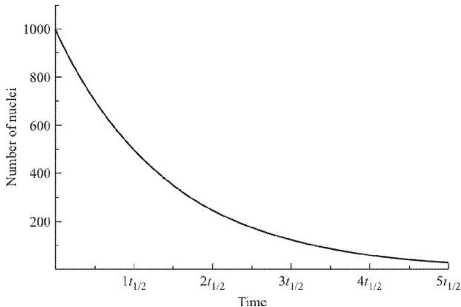
**Figure 3.2** Exponential decay curve for  $^{24}\text{Na}$ .
