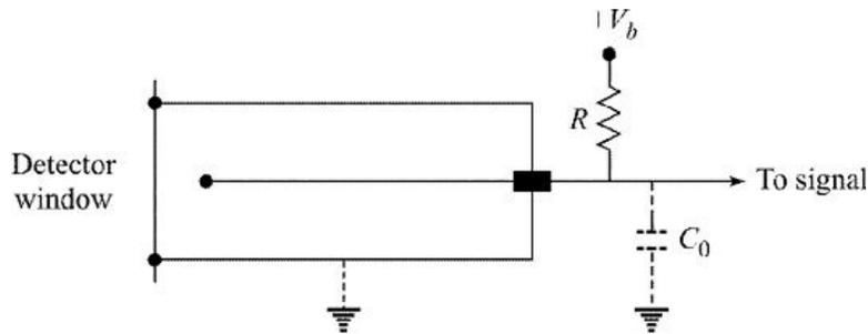
Figure 7.5 Schematic diagram of a proportional counter.
