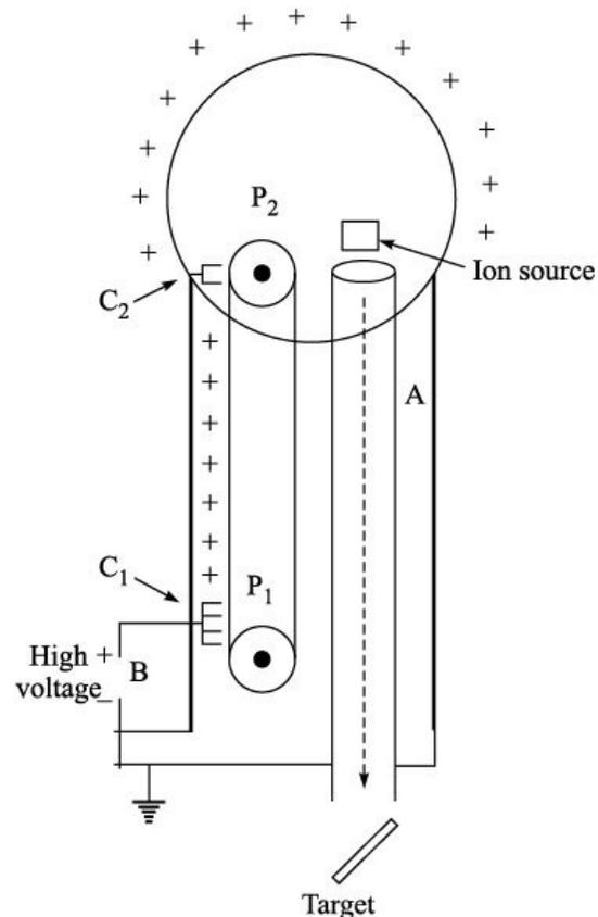
**Figure 6.2** Schematic diagram of Van de Graaff accelerator.
