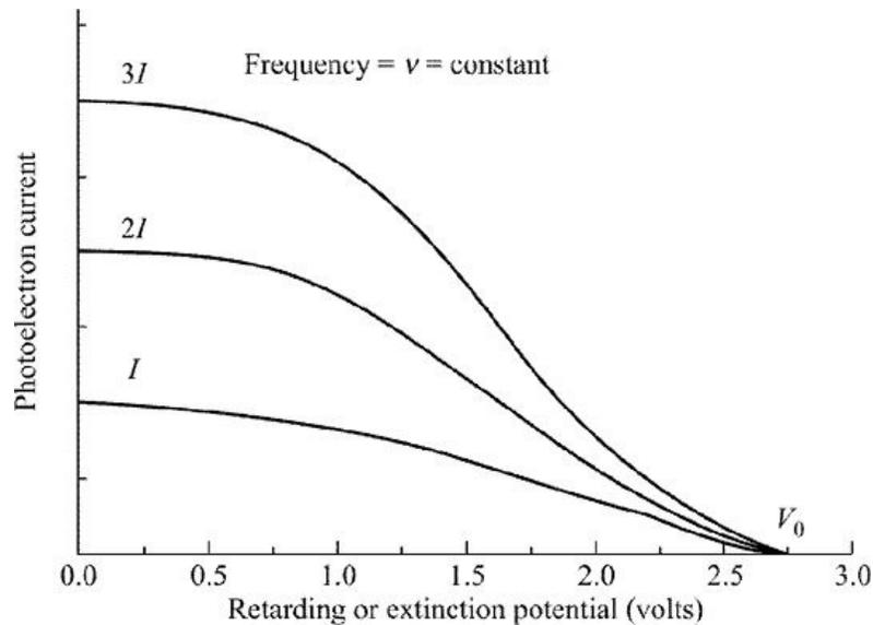
**Figure 5.6** Photoelectric current versus retarding potential for various intensities of incident light.
