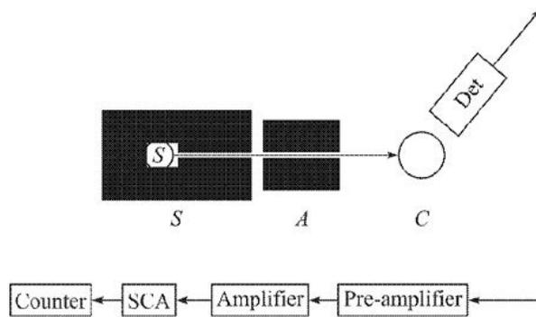
**Figure 5.9** Experimental set-up to verify Compton effect.
