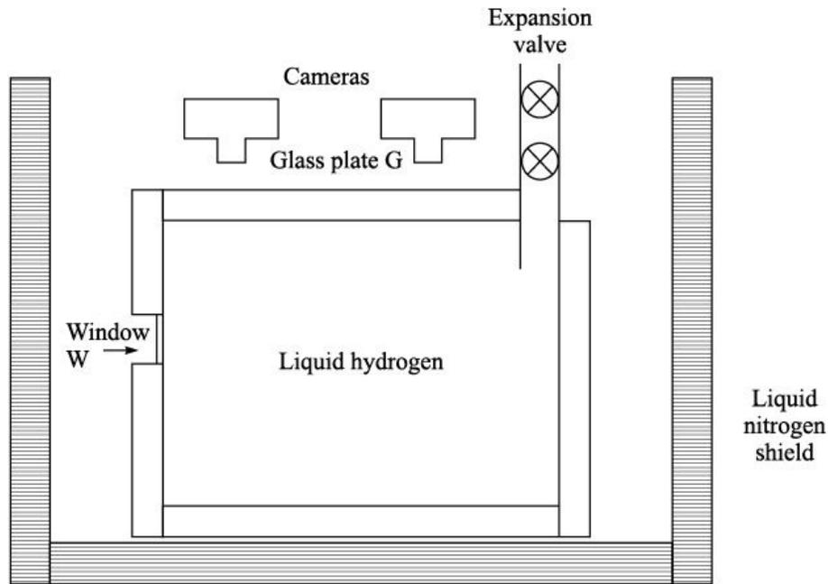
**Figure 7.20** A schematic diagram of bubble chamber.
