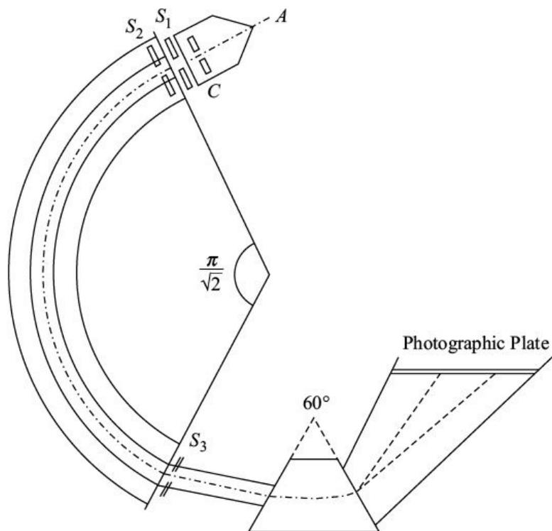
**Figure 1.10** Schematic diagram of Bainbridge and Jordan mass spectrograph.
