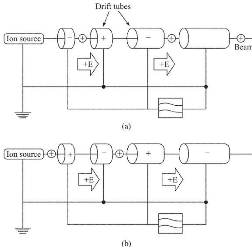
**Figure 6.4** (a) the first drift tube is negatively charged. It means beam of +ve ions will be accelerated, (b) the first drift tube is positively charged. It means beam of +ve ions will not be accelerated.
