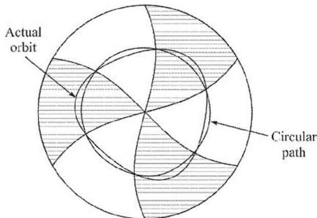
**Figure 6.12** High-field and low-field regions in an A.V.F. cyclotron. Particles perform radial oscillations
