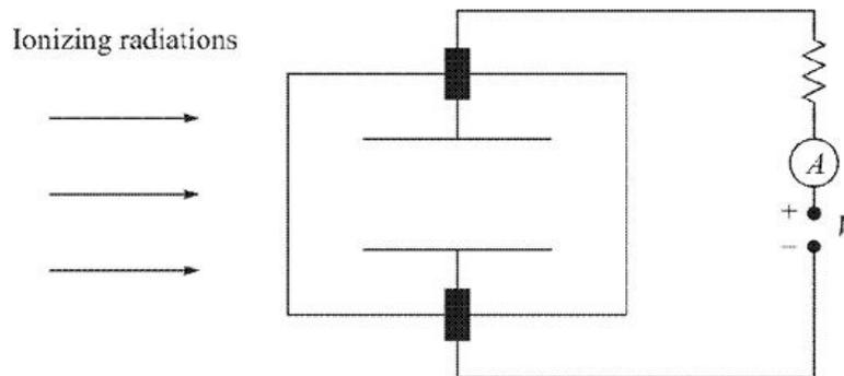
Figure 7.4 Ionization chamber.
