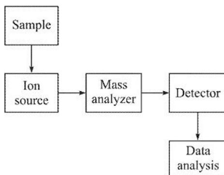
**Figure 1.8** Block diagram of the mass spectrometer.
