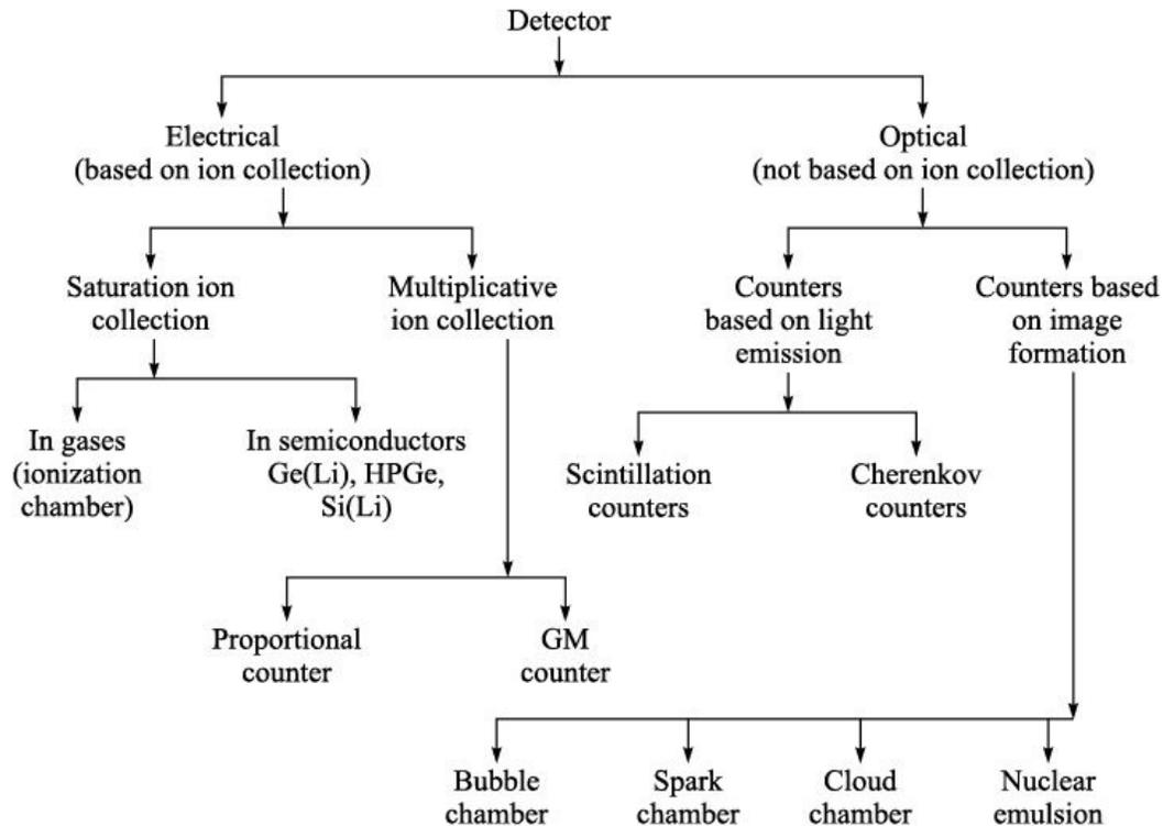
**Figure 7.1** Classification of detectors according to signals produced.
