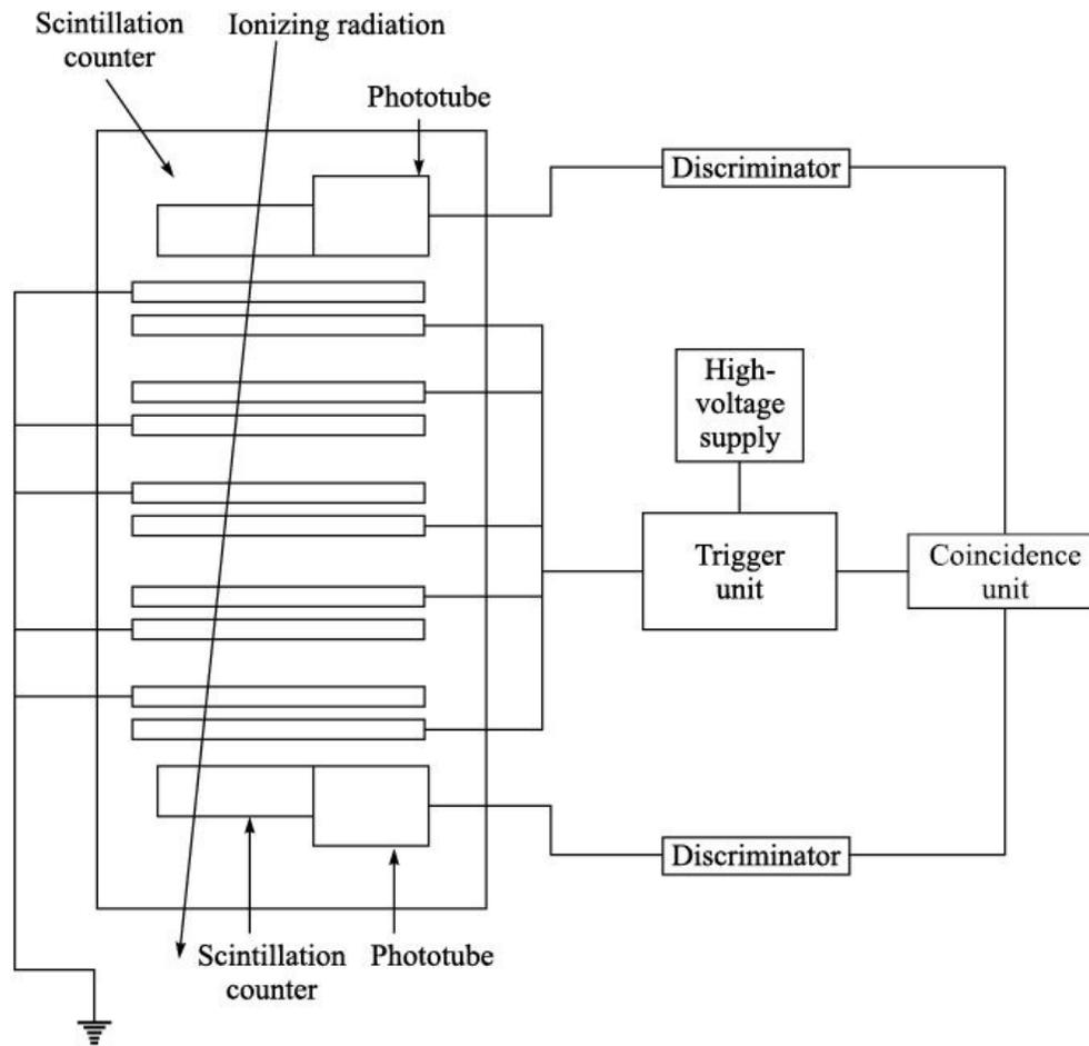
**Figure 7.21** Spark chamber.
