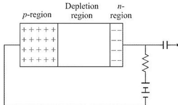
**Figure 7.14** Reverse biased diffused  $p$ - $n$  junction.
