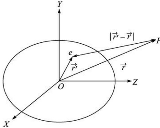
**Figure 1.5** Non-spherical charge distribution. The nuclear charge  $e$  is located at a distance  $r_{\text{ns}}$  from the origin and the potential at point  $P$  outside the nucleus at a distance  $r_{\text{ns}}$  from the origin.
