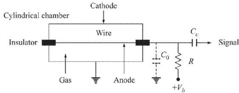
**Figure 7.2** Schematic diagram of a gas-filled detector.
