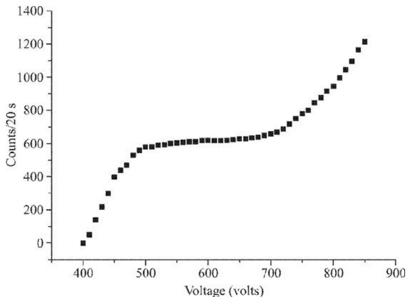
**Figure 7.8** Plateau curve of a GM counter.
