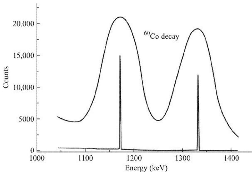
Figure 7.18 Comparative *g*-ray spectrum of  $^{60}\text{Co}$  as recorded by Ge(Li) and scintillation [NaI(Tl)] detectors.
