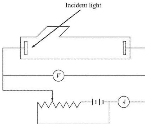
**Figure 5.5** Set-up used for verification of photoelectric effect.
