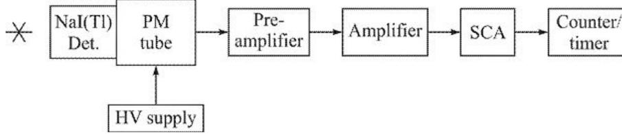
**Figure 7.10** Block diagram of a scintillation spectrometer.
