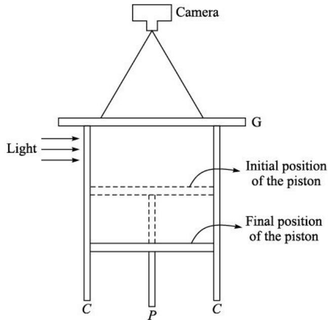
**Figure 7.19** A simplified diagram of cloud chamber.
