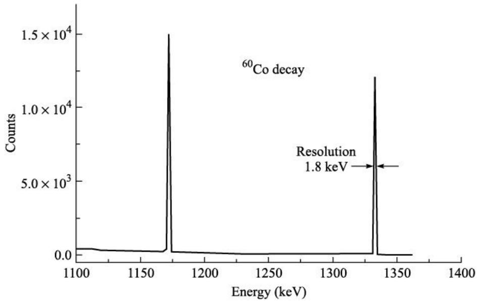
Figure 7.17 *g*-ray spectrum of  $^{60}\text{Co}$  as recorded by Ge(Li) detector.
