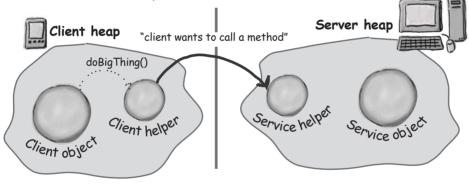
Service helper unpacks the information from the client helper, finds out which method to call (and on which object) and invokes the <u>real</u> method on the <u>real</u> service object.
