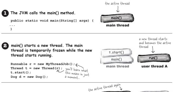
The JVM switches between the new thread (user thread A) and the original main thread, until both threads complete.
