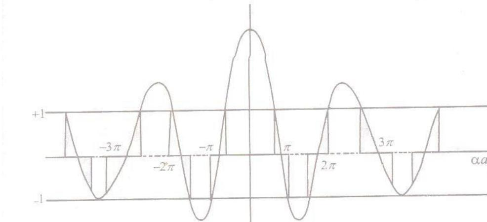
Plot of the left hand side of eq (4) as a function of  $\alpha a$  for  $p = \frac{3\pi}{2}$ . The solid and broken lines on the abscissa ( $\alpha a$ - axis) correspond to allowed and forbidden energy regions of the energy spectrum respectively that are plotted in fig.
