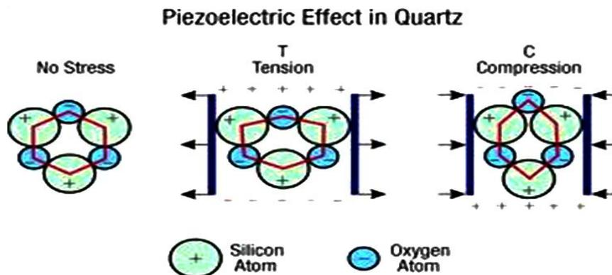
*Fig. Piezo electric effect in quartz crystal*
