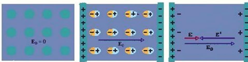
Fig. (a) non polar dielectric in  $E=0$  (b) Non polar dielectric when 'E' is applied
