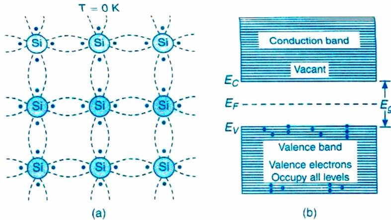
*Intrinsic silicon crystal at  $T=0K$  (a) 2-D representation of silicon crystal
