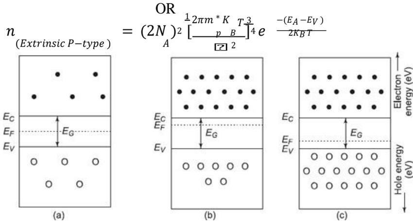
Energy band diagrams of (a) Intrinsic semiconductor (b) N- type & (c) P- type semiconductors
