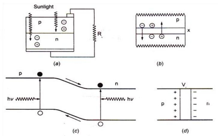
Fig. (a) p-n junction solar cell with load resistance,  $R_L$  (b) Diffusion of electrons & Holes (c) Energy band diagram of solar cell (d) Formation of the open circuit voltage  $V_0$
